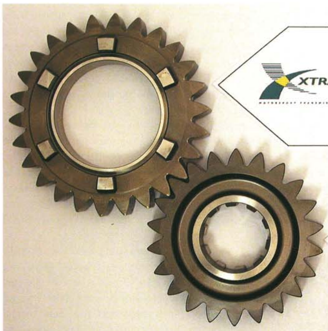
A 22:26 gear ratio set from the early 1990s, in carburised re-melted steel
