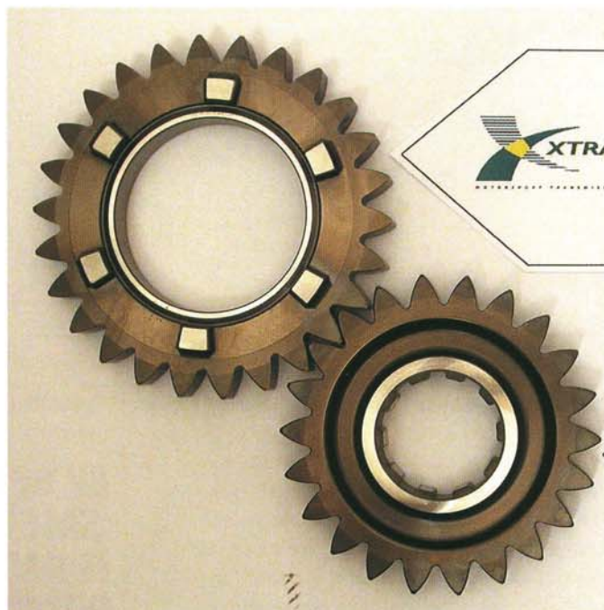
Same gear ratio set, mid-1990s – by now around 2mm narrower in width
